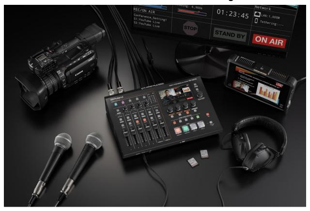
Easy-to-use enterprise solution that combines a video switcher, audio mixer, preview screen, recorder/player, and streaming encoder in one portable unit.
